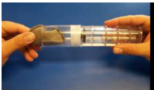
Step 4: Install bean bag, squash ball or up to nine paint ball markers. Wet squash ball to help install into cartridge.
