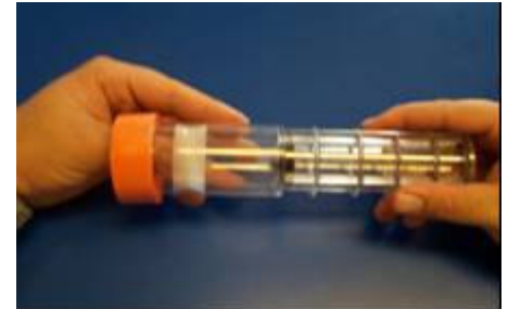
Step 3: Push piston past install tool into the cartridge. Remove tool and continue to push piston until it bottoms out in cartridge.
